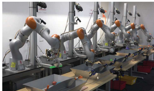
Fig. 3. Large-scale data collection setup consisting of 8 Kuka IIWA robots, used to evaluate transfer learning after another setup was used to collect a dataset consisting of over 800,000 grasp attempts [29].
