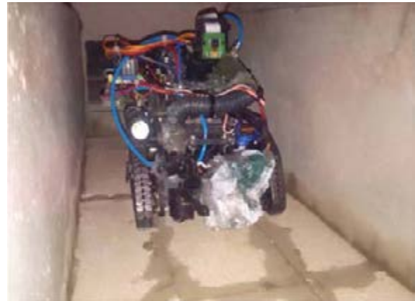
Figure 7. Tread driven movement in air duct
