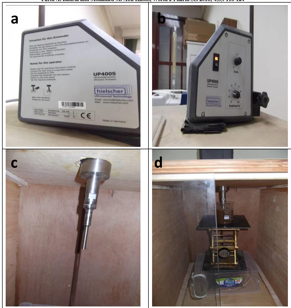
Fig.4: Direct sonication device (Hielscher UP400S ultrasonic processor, 24 kHz) a: left side view of the device b: right side view of the device c: Horn tip of the direct sonication device d: Extraction process with direct sonication placing the horn tip inside 250ml beaker containing plant material with the solvent.
