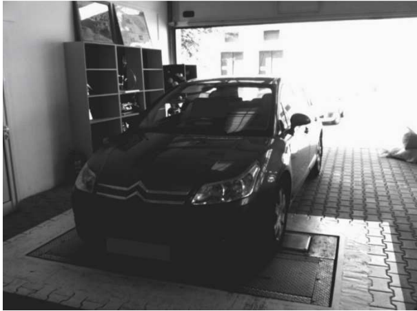
Fig. 1. Determination of the load on the front axle using the tool with the scales.
