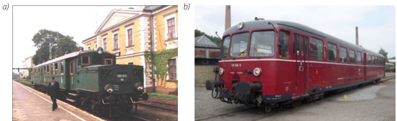
Fig. 1. Battery-powered trains in 20th century: a) the only existing Wittfeld train, designation Ma 090 802 [2], b) battery-powered railcar, DB Class ETA 150 [5]
