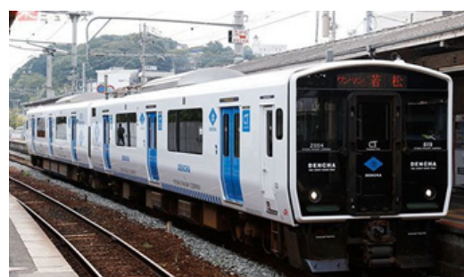
Fig. 3. EMU with energy storage, BEC819 series [8]
