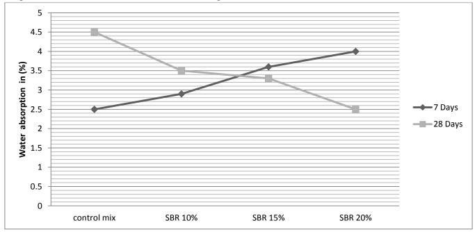
Figure 3: Water Absorption of Mix containing same percentages of "RIPSTAR 148"-latex
