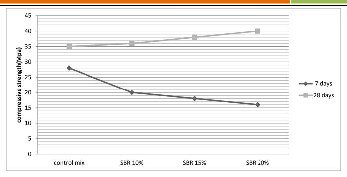
Figure 2: Compressive Strength of Mix containing same percentage of "RIPSTAR" 148-latex
