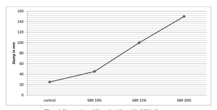
Figure1:Slump values of Control and Latex Modififide Concrete
