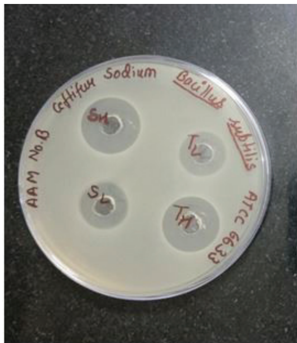
Fig. 2: Two level agar diffusion assay method using a test microorganism Bacillus subtilis ATCC-6633 (MTCC 441) at concentration of Reference solution S_H = 4 \mu\text{g mL}^{-1} , S_L = 1 \mu\text{g mL}^{-1} and Sample solution S_H = 4 \mu\text{g mL}^{-1} , S_L = \mu\text{g mL}^{-1} .
