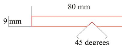
Fig. 1. Geometry of IZOD sample
