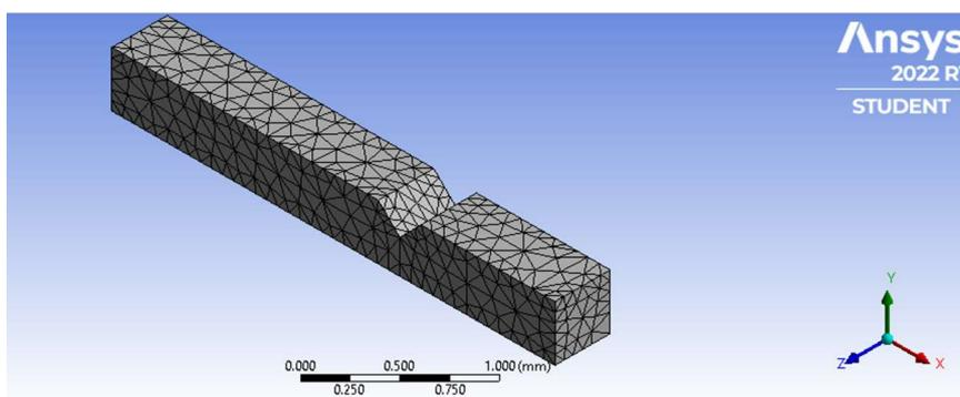
Fig. 2. The meshed model
