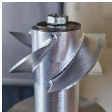
Fig. 3 Pump inducer under manufacturing
