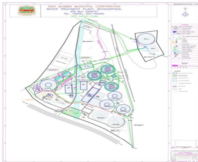
Figure 2: Layout Plan of Water Treatment Plant
