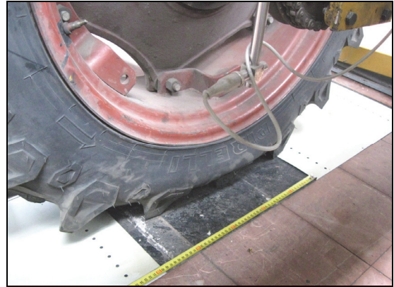
Fig.4. Measuring tyre contact length
