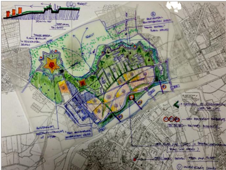
Fig.5. Conception draw showing increased to 6 (two available) the possibility of crossing the river (mostly walkways, bridge for pedestrian and bicycle traffic), explaining the opportunities for the revitalization of investment terrain after the ZSD factory, with the activation of pathways in the direction of forts to the north.
