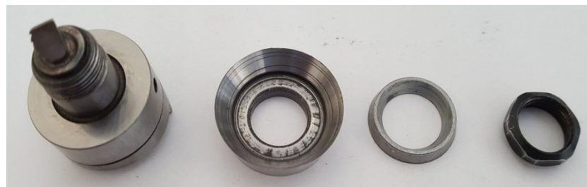
Figure 5. Elements of blade inserts with fixing elements
