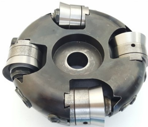
Figure 3. Standard milling head based on self-rotating blades
