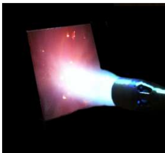
Figure 13 The bare steel plate during the fire performance test.
