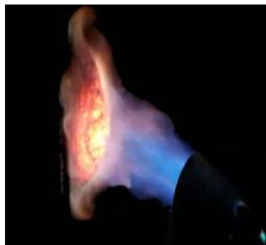
Figure 15 The steel plate coated with IFR-F3 during the fire performance test.
