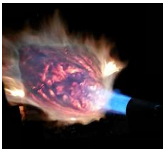
Figure 14 The steel plate coated with IFR-F2 during the fire performance test.
