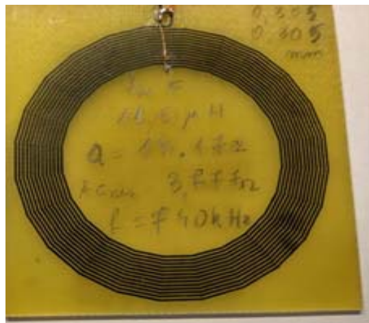
Fig. 8. Wireless power transfer inductor made with WEBENCH Coil Designer online tool using the manual toner transfer method for validation and testing purposes.
