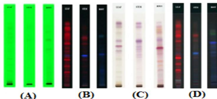
Fig. 1: The fig. of developed TLC plates under UV-254 nm (A) and UV-366 nm (B), under white light after derivatization with ASR (C) and under UV-366 nm after ASR (D) for 10 µl sample size
