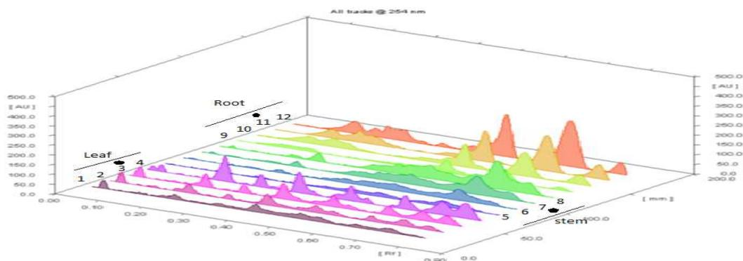
Fig. 2: The fig. of densitogram results of developed TLC plate under UV-254 nm. Densitogram was showing 2 µl, 5 µl, 10 µl and 20 µl scanning results of leaf (track 1,2,3,4), stem (track 5,6,7,8) and root (9,10,11,12) extracts respectively from left to right, while the star pointed tracks (track 3, 7, 11 for leaf, stem, and root respectively) were standard optimized 10 µl sample volume tracks which were used for final densitogram studies for fingerprinting method development
