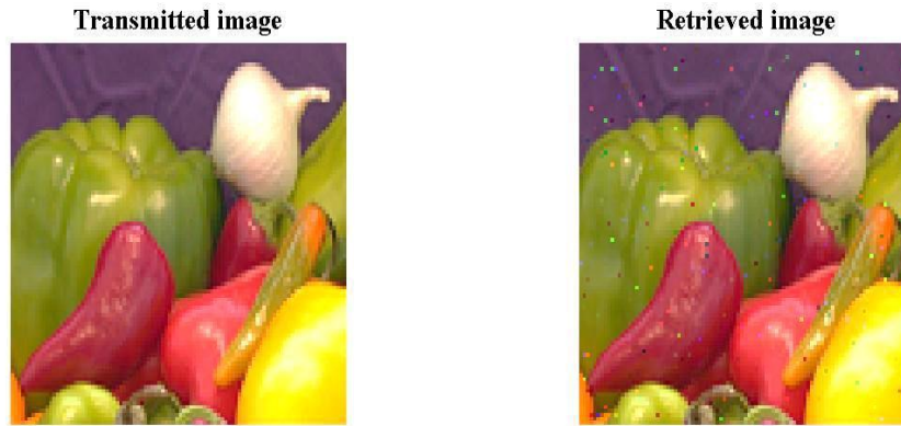
Figure 6: Performance indicator of MGSTC BLAST spatial multiplexing scheme aided MCCDMA wireless communication system under implementation of MMSE-SIC signal detection, 16-QAM digital modulation for a typical image at SNR value of 3dB
