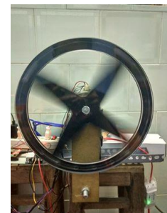
Fig. 7. RWIP model when being stable..
