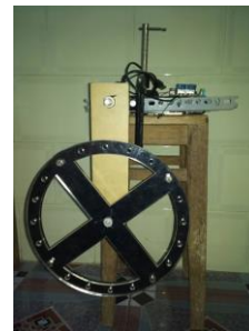
Fig. 6. RWIP model when being unstable.
