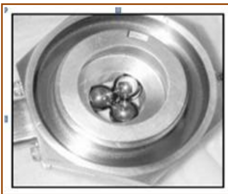
Fig. 1 Three balls are locked into base fixture
