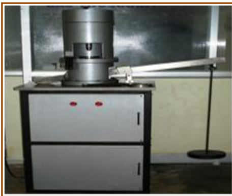
Fig. 4 Loading arm connected with four ball tester to measure wear
