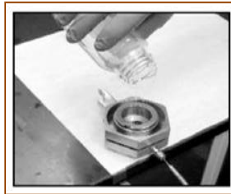
Fig. 3 Test lubricant is poured into the base fixture
